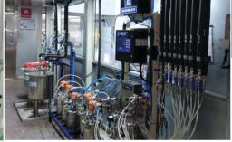
Patvin has for many years delivered both manual and automatic 2K painting systems to the surface treatment industry. With intrinsically safe fluid panels, the systems easily integrates into hazardous areas, single or multi-color and catalysts.
